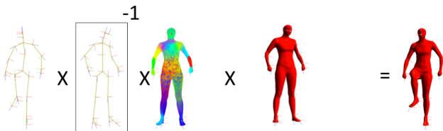
Figure 3: Visualization of linear mesh blending. From left to right: target pose, template pose, weights, template mesh, and target mesh. The final vertices position vector \mathbf{p}(\mathbf{q}) is calculated by weighing vertex position w.r.t. transformations of a few joints applied to the template vertex position.
