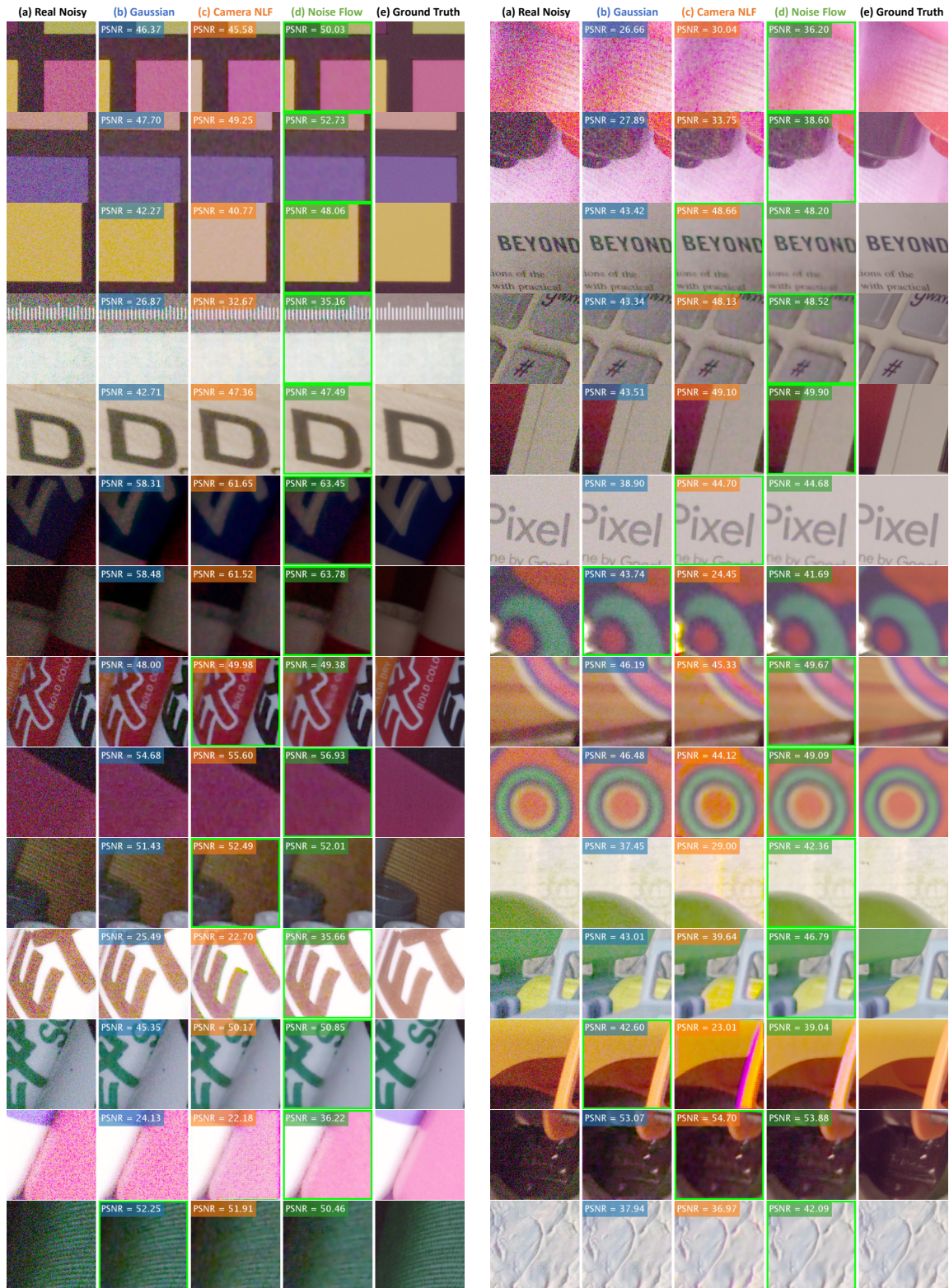
Figure 3: Sample denoising results from the DnCNN denoiser trained on three different noise synthesis methods:(b) Gaussian; (c) camera NLF; and (d) Noise Flow. (a) Real noisy image. (e) Ground truth.
